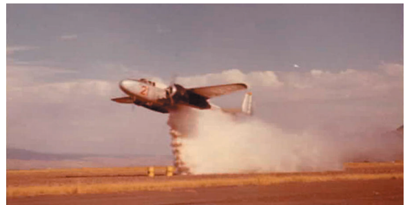
B25 performing test of simulated borate at La Grande airport
