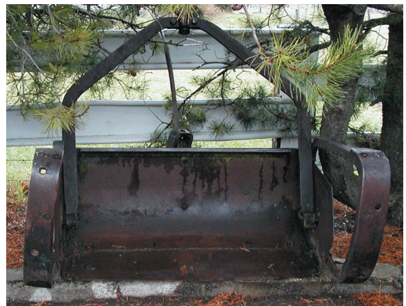
A fresno--metal dirt scraper, formerly drawn by horses and guided by a man; used in making roads, for example
